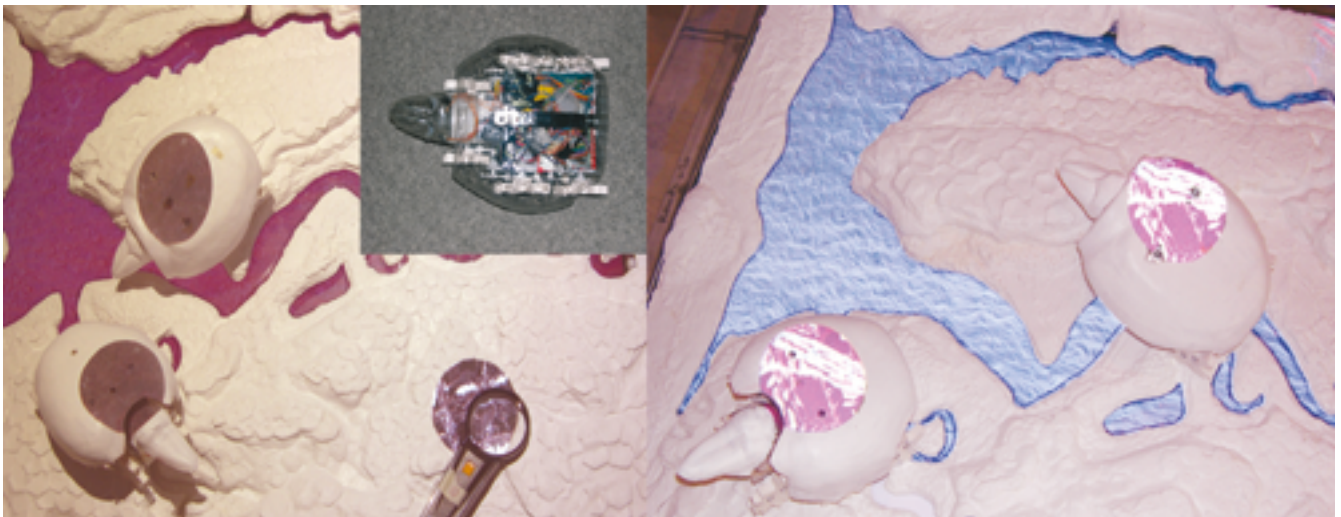
THE ROBOTS IN DERMALAND MOULDED ON DUSTMITES/WEEVILS AND BUILT USING OPTICAL AVOIDANCE DIY 2WD ARDUINO KITS.
